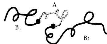
Figure 2. Schematic representation of an asymmetric B 1 -A-B 2 triblock copolymer, where B 1 and B 2 are chemically identical blocks differing only in molecular weight.
